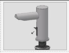
Connect the motor connector to its matching connector coming from the electronic unit. Please note that since the connector is water proof, some friction might apply.
