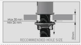
If your dispenser is supplied with anti-rotation solution, drill an additional hole for anti-rotation pin.
